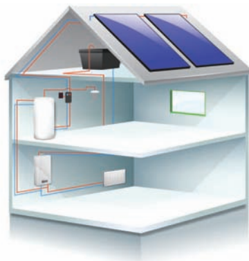
Zenith Solar system Mynute VHE regular open vent boiler Aquaflow Twin coil cylinder
