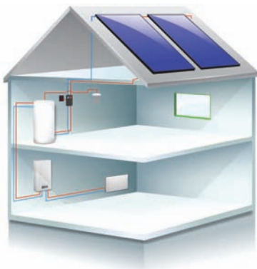
Zenith Solar system Mynute HE sealed system boiler Aquaflow Twin coil cylinder
